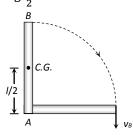
When it strikes the floor, its potential energy will convert into rotational kinetic energy
