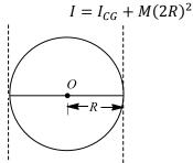
where,  $I_{CG}$  is moment of inertia about an axis through centre of gravity.
